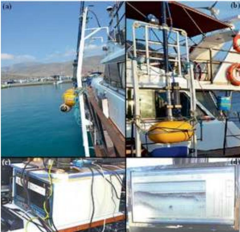
**Fig. 9.77** (a, b) O.R.E. Model 132A/132B over-the-side Transducer Mounting (c) Universal Transceiver of the chirp system and (d) a chirp seismic profile collected from the surveyed area (Photo courtesy G. Papatheodorou, University of Patras)
