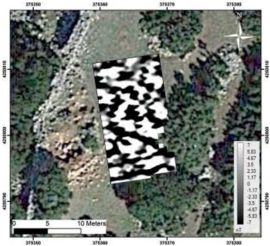
**Fig. 9.28** Distribution of the magnetic gradient in the area of the cells K1 and K2. This bit of land is in contact with the open pit that revealed the Mycenaean tomb at the western side of the hill of Kastrouli. The gradients are clipped to the range  $[-7,7]$ nT/m. The satellite picture of Google Earth has been used as background
