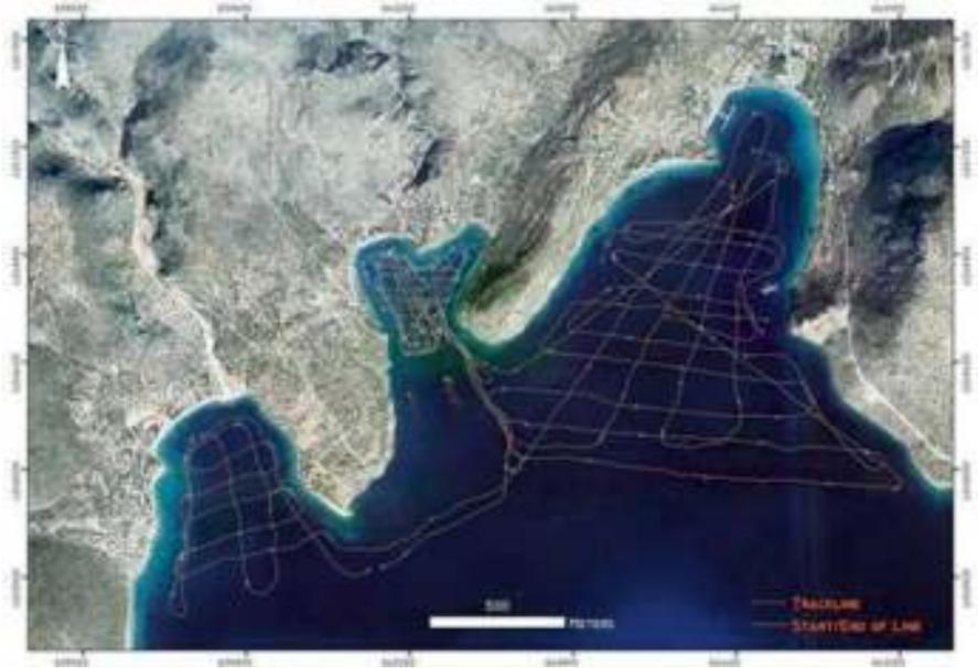
**Fig. 9.74** Map of the surveyed areas showing the tracklines of the side-scan sonar and sub-bottom profiling. From right to left – Ag. Isidoros, Potami/Ag. Sotirios, and Valtos (Photo courtesy G. Papatheodorou, University of Patras)
