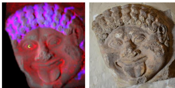
(Left) Chemical map of lead (green), iron (red) and copper (blue) showing the distribution of remains of pigments on the Medusa head. (Right) picture of the marble sculpture, Delphi, Greece.
