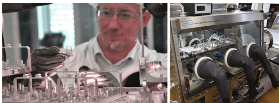
Fig. 3.11 Sample integration process using the EML glovebox
