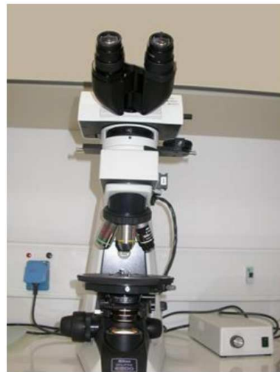
Figure 1. Polarized light microscopy (PLM) with various components (© lab of archaeometry, University of the Aegean, Rhodes).
